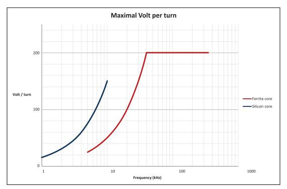
For lower frequencies it is possible to get the MT with Silicon Iron core, and/or with double the windings in the primary.
